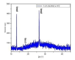
**FIGURE 1.** Powder XRD patterns of Mn doped BMZ films deposited for 5 wt % at 50 °C.
